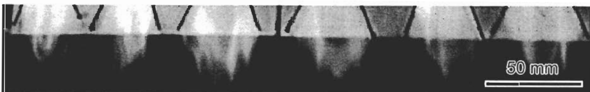
Fig.9 Photograph of 6 channel discharges of multi-gliding arc plasma.
